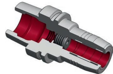
**Application:** High precision clamping of cutting tools with cylindrical shank DIN 6535 form HA, HB, HE and tool shanks according to DIN 1835 form A, B with shank tolerances h6.
