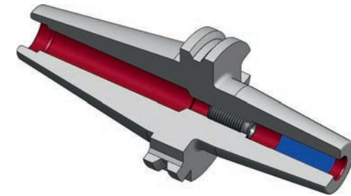
**Application:** Quick and safe clamping of tools with cylindrical shank. Thanks to the patented relieved bore (from 6mm diameter), you can shrink even more quickly and precisely. Ideal for HPC and HSM milling.
