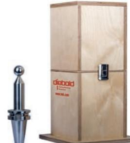
**Test arbor for testing RTCP (Rotation Centre Point) of 5-axis spindles.**
