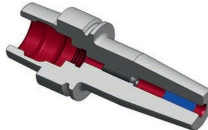
For automatic tool change, central coolant through.
