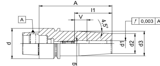
**HSK ShrinkFit Chucks**
