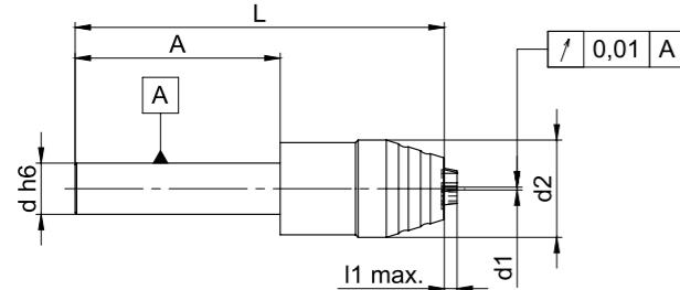
**Micro Drilling Chuck with Straight Shank**
