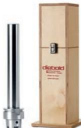
To check the runout of HSK spindles.
