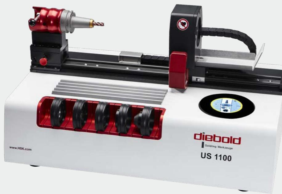
*Diebold offers various types of shrink units. From small devices for shrinking micro-tools to large devices for shrinking tools for heavy-duty machining. The larger units have an integrated water cooler for automatic cool-down.*
