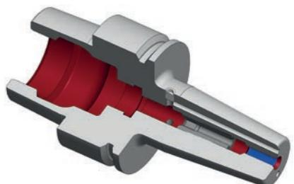
For automatic tool change, central coolant through.
