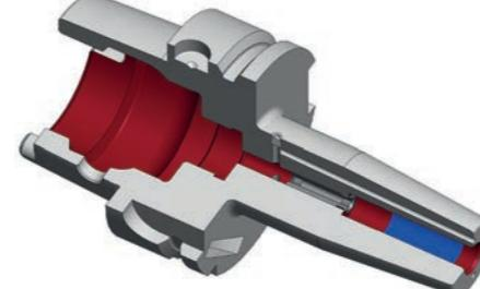
**Application:** Fast and secure clamping of tools with cylindrical shank. Easy handling by relieved bore (starting from Ø6mm). Ideal for high RPM applications like HPC and HSM.
