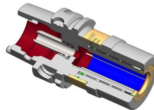
**Application:** Highest gripping force. Perfect for heavy duty milling. With Jetring for internal cooling.
