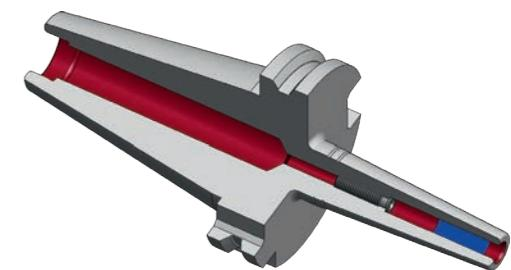
**Application:** Quick and safe clamping of tools with cylindrical shank. Thanks to the patented relieved bore (from 6mm diameter), you can shrink even more quickly and precisely. Ideal for HPC and HSM milling.
