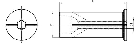
Reductions for UltraGrip™ and UltraJet™ Chucks and Hydraulic Chucks – with coolant slots
