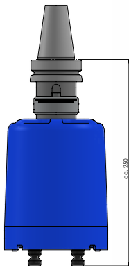
Workholding hood with BT 40
