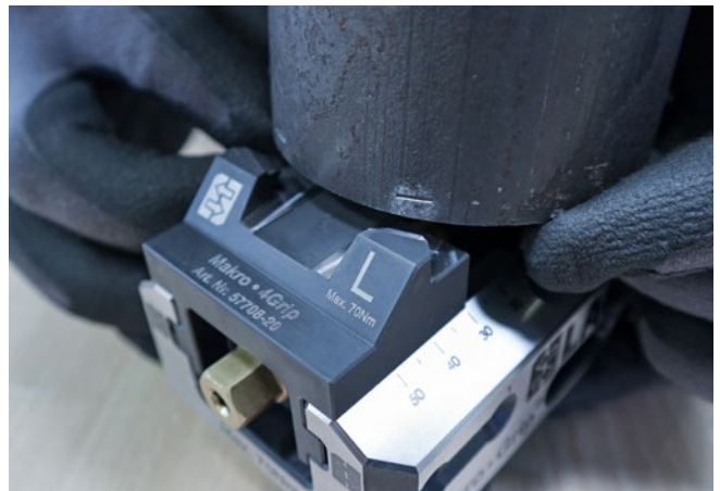
The clamping jaws grip the pre-stamped workpiece in four indentations.
