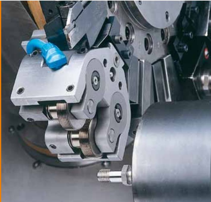
WAGNER® thread rolling attachment rolling threads in front of a collar
