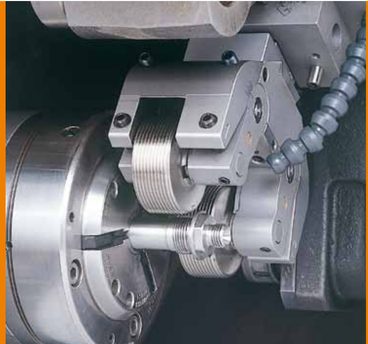
Thread rolling behind a collar
